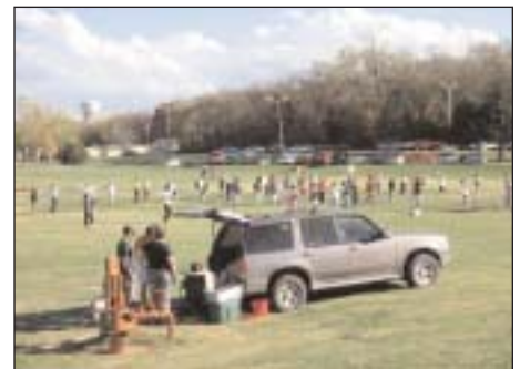
Ground water sampling to the tune of "Fight on Emporia." Field chemical parameters are measured in monitoring wells (behind the vehicle) during an aquifer test. The nearby floodplain margin (tree-covered terrace in background), allows for evaluation of boundary effects during data interpretation.
