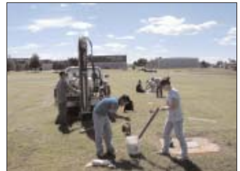
Soil samples are obtained in Environmental Field Methods class using direct-push tools. Forty feet of continuous core were laid out in the foreground for description and sampling, while monitoring wells are installed in the background. Soil sampling and well drilling activities were made possible through collaboration with Larsen and Associates Inc. and Hydrologic Inc. The interaction with local professionals provides students with exposure to career options in hydrogeology.
